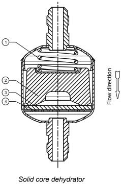
1 - Spring 2 - Bock 3 - Felt 4 - Stainless steel mesh
